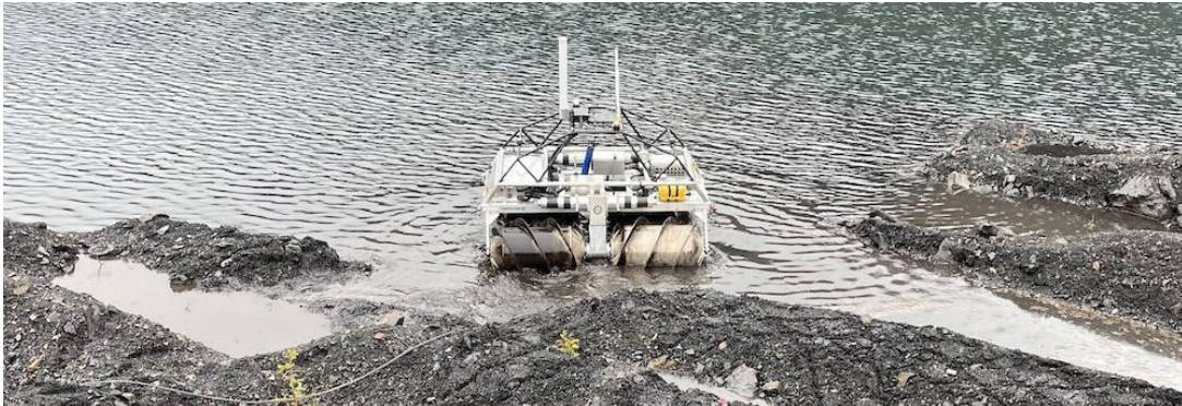
Figure 8: HELIX Neptune deployed in a pit-lake with YSI EXO Sonde
