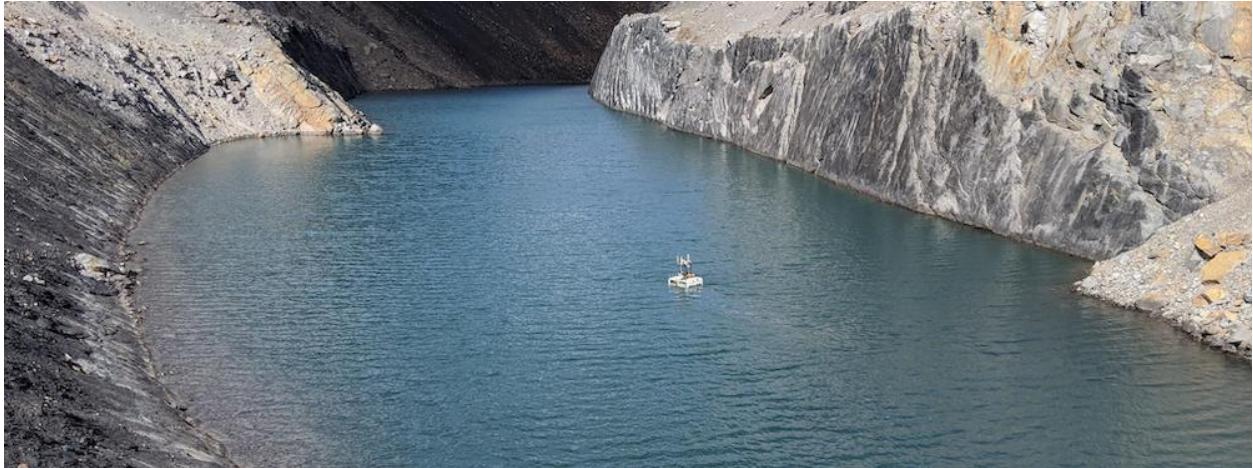
Figure 6: HELIX 25 conducting a bathymetry survey in a pit-lake
