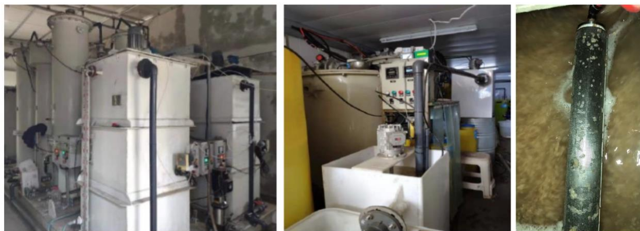
Figure 3: Photograph of the pilot plant equipment, CIF® (left), BIOCLENS® reactors (middle), self-cleaning screen (right)
