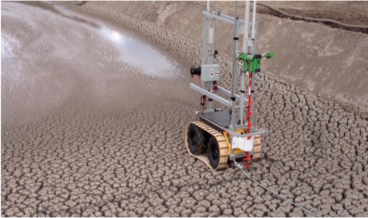
Figure 4: RTC-II UGV drilling on an oil sands tailings deposit
