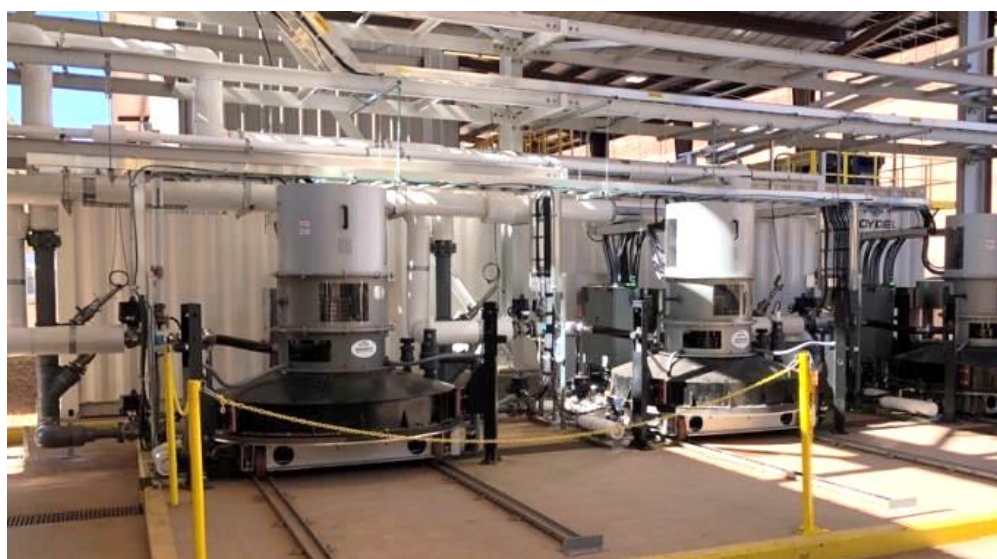
Figure 7: ERC with constant-gap electrocells applied to NF retentate
