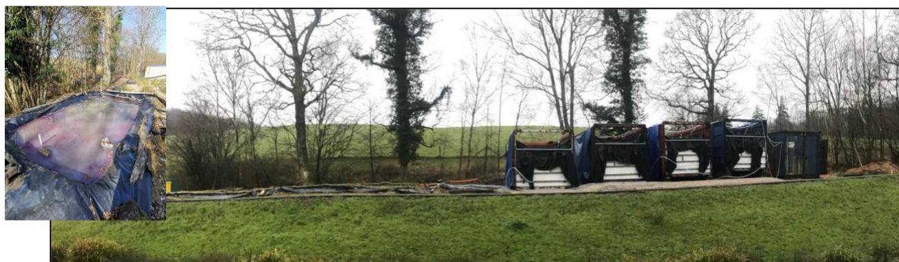
Figure 6: Passive treatment pilot plant from right to left (feed tank; BCR1, 2, 3, 4; reed bed (APW) 1, 2, discharge holding pond showing purple/white bacteria)
