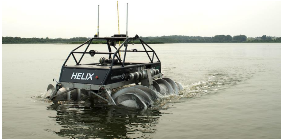
Figure 5: Screw-drive amphibious robot moving across a lake
